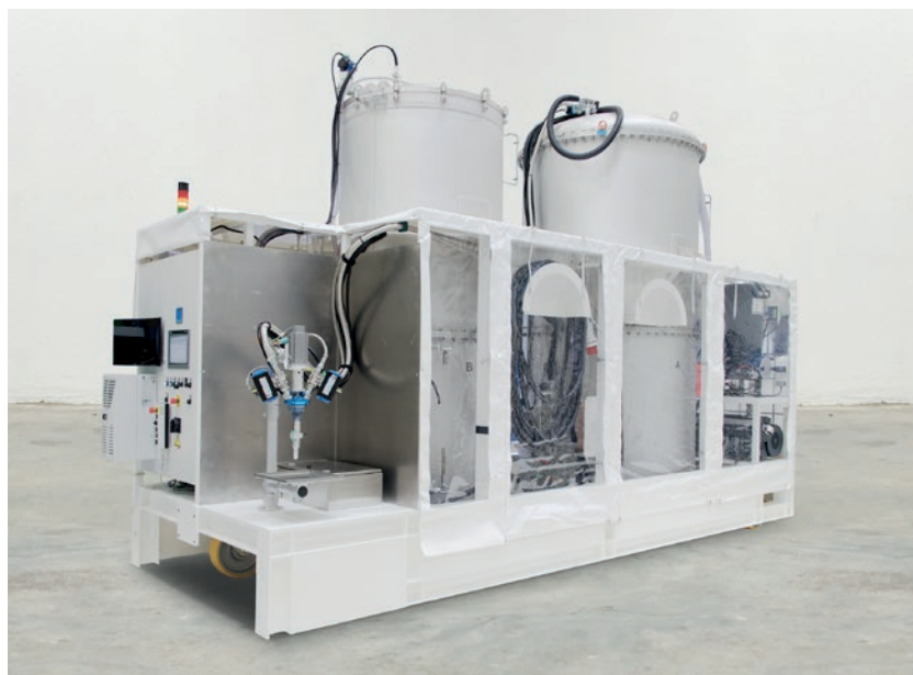
Ready for the vacuum infusion: Large Nodopur plant from TARTLER with integrated degassing unit for processing low-viscosity epoxy or polyurethane resins and hardeners in rotor blade production.
