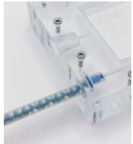
The filling of the mold can start. The material flow opens the Flowstop.
