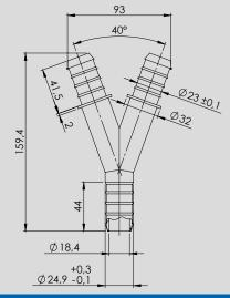
Y-connector for 25 mm hoses: Sketch with dimensions and diameters
