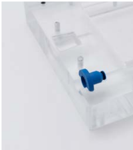
Place the Flowstop in an open mould, then reclose the mould.
