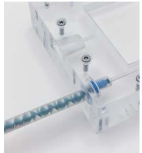
The filling of the mould can start. The material flow opens the Flowstop.
