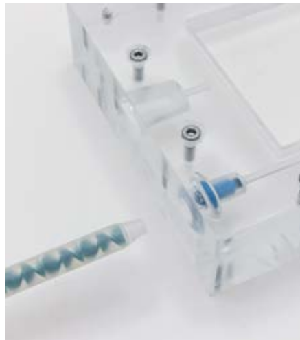
The mixer sleeve is shortened at the front and inserted into the Flowstop until it meets with resistance.
